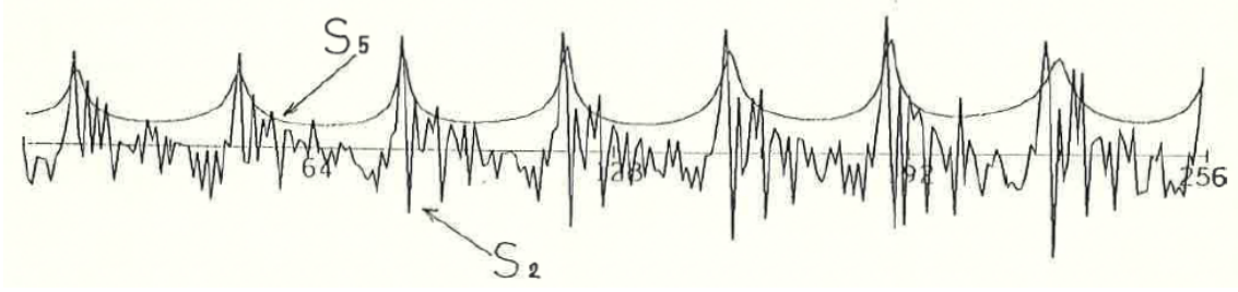
Figure 2.6: Residual signals and the amplitude envelope signals.
